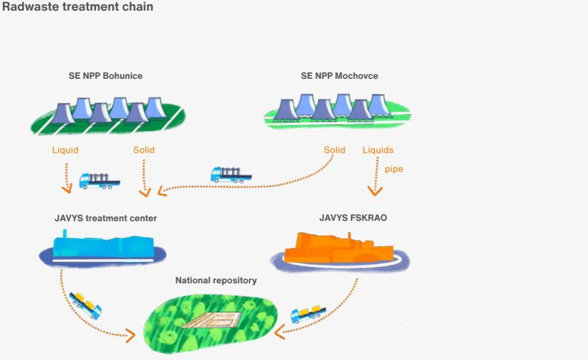
FSKRAO: final processing of liquid radioactive waste
